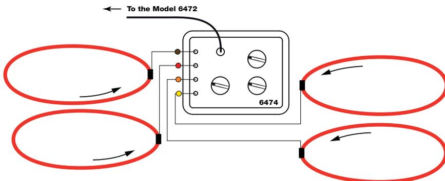
4. On the Model 6474, set the **INPUT** selection switch accordingly. You can measure the current flowing through one GroundFlex® sensor (1, 2, 3, or 4), or through several sensors (1, 2 or 1, 2, 3), or through all of the sensors (1, 2, 3, 4).
