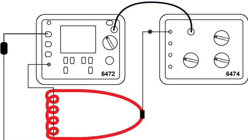
1. Set the switch of the 6472 to **SET-UP**.
