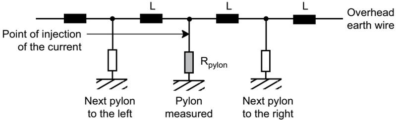
A measurement in SWEEP mode of an installation like this having 10 towers gives the following results assuming an earth resistance  $R_{pylon}$  of  $10 \Omega$  for each tower and an inductance  $L$  of  $550 \mu\text{H}$  for the link via the overhead ground conductor at the tip of the towers:
