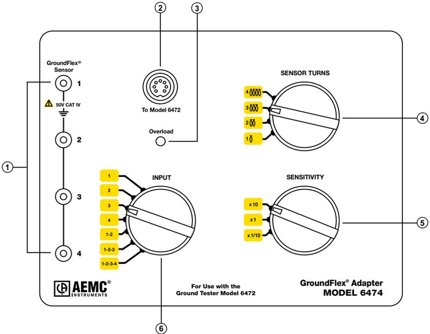
1. Inputs 1 through 4 for GroundFlex® sensors
