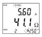
Display of the **NOISE** symbol during the impedance measurement indicates that the current (> 5 A) or voltage (ZxI > 25 V) is too high, making the accuracy of the displayed measurement uncertain.
