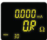
Indicates that the impedance is greater than 1500  $\ensuremath{\Omega}$
