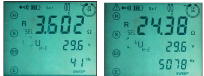
Sweep Test Results (low frequency [41Hz] on left, high frequency [5078Hz] on right)
