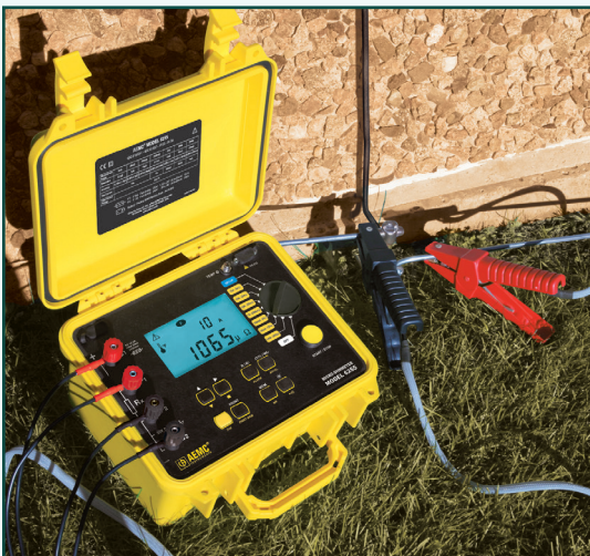
Model 6255 conducting bond verification on a grounding system.
