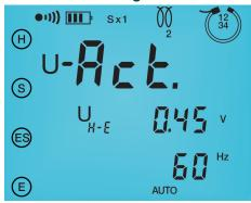
Live voltage is measured between the tower and the measurement auxillary electrode to ensure accurate testing by verifying the electrodes distance is sufficient.
